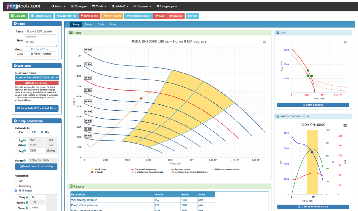
Figure 11 . Well “9” ESP upgrade design with the PumpDesign tool
