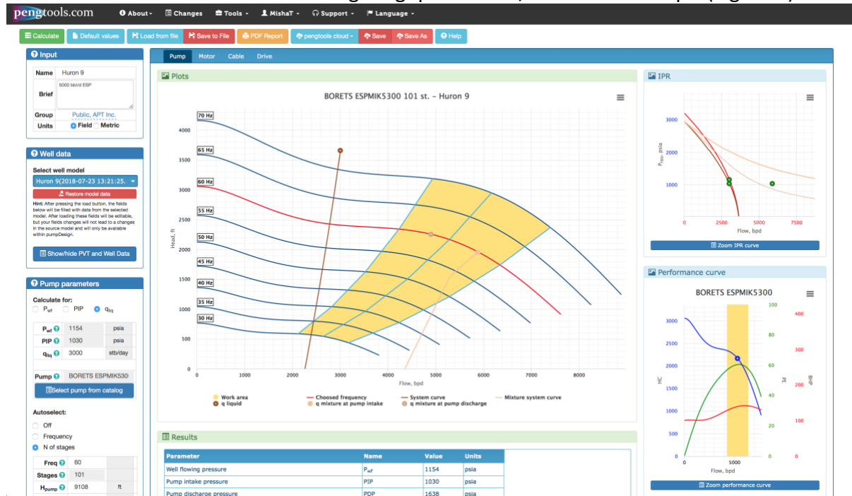
Figure 9 . Well “9” ESP design with the PumpDesign tool
